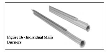
Clean individual burners using air pressure or soft brush. Use an air nozzle to blow out scale and dust accumulation from the burner ports. **CAUTION: Wearing eye protection is recommended.** Alternately blow through burner ports and venturi. Use fine wire to dislodge any stubborn particles. Do not use anything that might change the port size.
