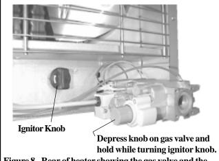
Figure 8 - Rear of heater showing the gas valve and the knob on the Piezo ignitor  $\,$
