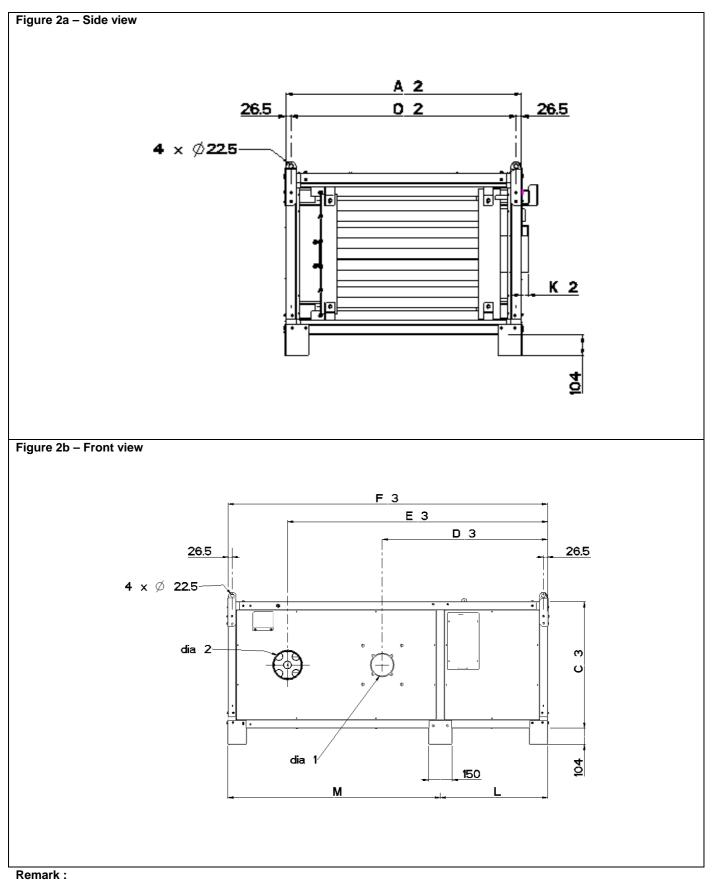
The fixation eyes (4x dia 22.5) may only be used to put the unit into horizontal position after delivery. It is strictly forbidden to use the fixation eyes for suspending the unit.
