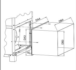
Attention must be given to the motor load when applying discharge ducting. Duct outlets must be adjusted when necessary to meet the values mentioned in table 9.
