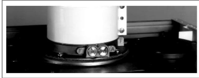
Using the especially designed apertures, readings can be taken on the temperature of the combustion by-products and of the combustion air, as well as of the concentrations of O<sub>2</sub> and CO<sub>2</sub>, etc.
