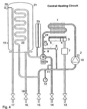
Main Heat Exchanger Automatic Air Vent Burner Ignition Electrodes Flame Sensing Electrode Differential Pressure Switch
