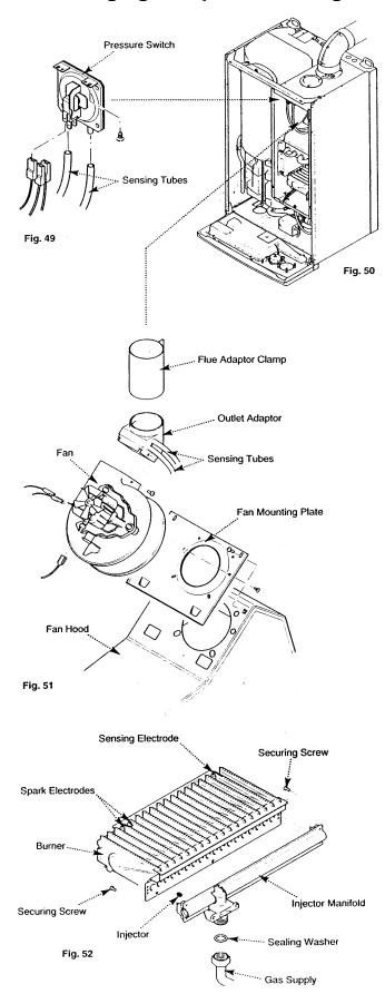
IMPORTANT: When changing components ensure that both the gas and electrical supplies to the boiler are isolated before any work is started.
