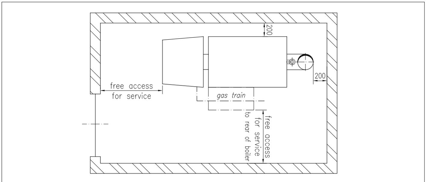
Fig. 04 Installation recommendations in the boiler house
