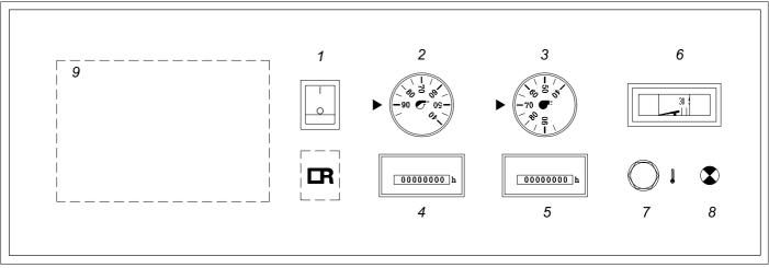
Fig. 09 Layout of the instrument panel High/Low with hours run meters 00.03F/79.00004
