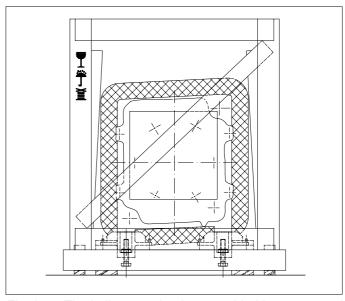
Fig. 05 The boiler completely assembled in a crate and on a pallet.
