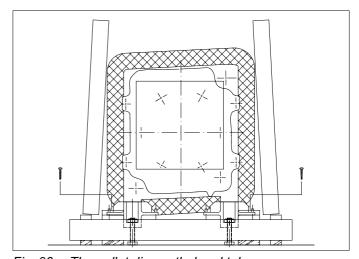
Fig. 06 The pallet dismantled and taken away 00.13C.79.00010, afb 2
