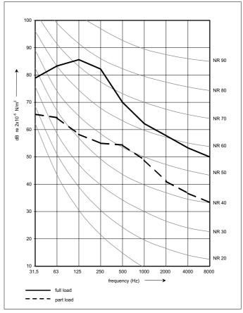
Fig. 03 Noise level readings without burner silencer
