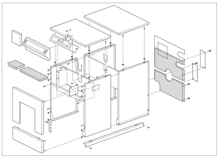
Fig. 08 Mounting casings and the instrument panel.
