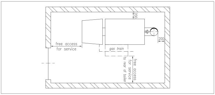
Fig. 04 Installation recommendations in the boiler house 04.15D.79.00001
