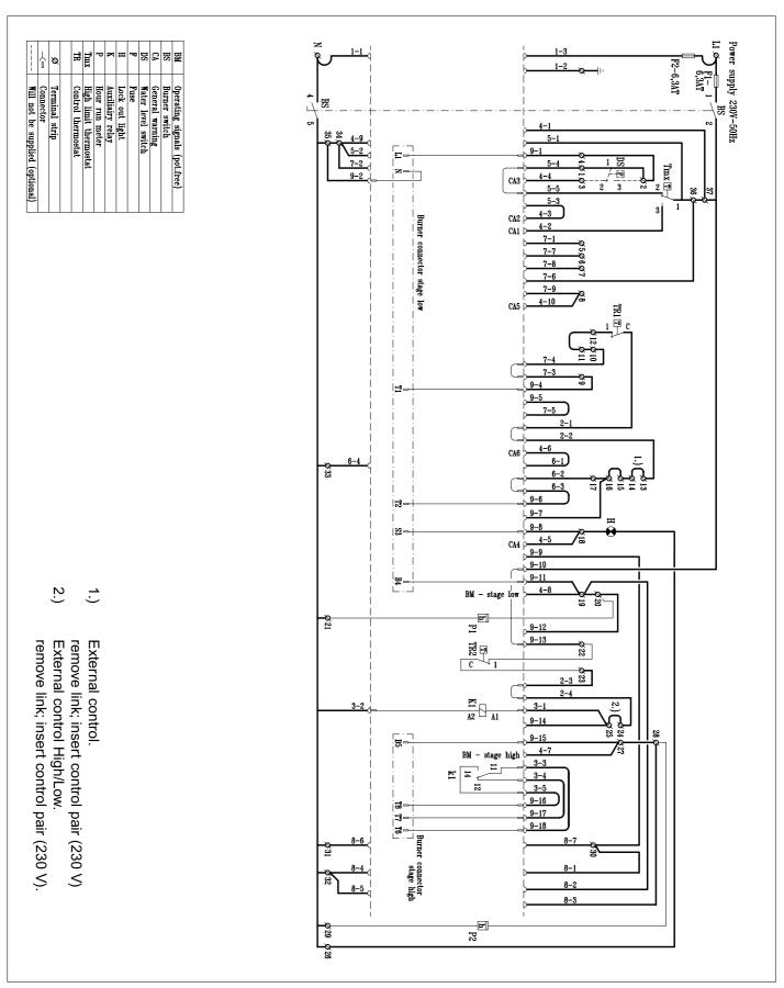
Fig. 10 Wiring diagram instrument panel High/Low with hours run meters
