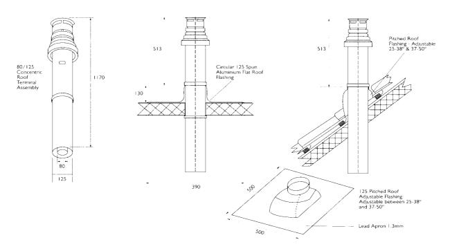
Concentric vertical flue fittings are available from eco hometec.
