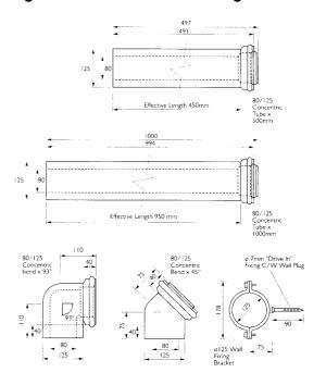
80/125 1000mm length PPS/White Galvanised Concentric Flue 80/125 500mm length PPS/White Galvanised Concentric Flue 80/125 PPS/White Galvanised 90 degree elbow 80/125 PPS/White Galvanised 45 degree elbow
