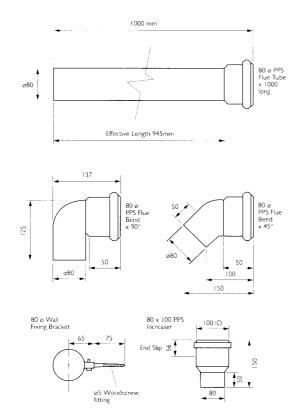
80mm 1000mm PPS flue pipe 80mm PPS 45 degree PPS Elbow 80mm PPS 45 degree connector 80mm Wall Fixing Clamp 80mm – 100mm increaser
