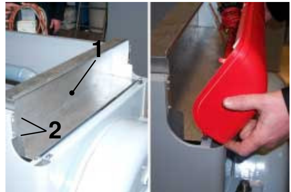
H Fit the wiring protection box "1" using the screws "2" on the sides, and position the pre-wired control panel.
