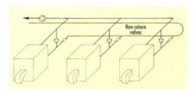
For traditional system operating on a  $\Delta t$  of 11°C then top flow (A1) and bottom return (A2) may be used although it is a mandatory requirement that a shunt pump is fitted and it is recommended that for circulation purposes a flow rate equivalent to  $\Delta t$  25°C is applied. Any shunt pump fitted must be proved running before the boiler is allowed to fire.
