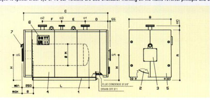
efficiencies in excess of 90% net. All PREXTHERM boilers are supplied with control panels that include control thermostat, high-low thermostat, limit thermostat (manual reset), hours run indicators for high and low fire, burner ON/OFF switch, burner lockout, thermometer and pressure gauge. All PREXTHERM boilers are CE approved and conform to the relevant European Standards.
