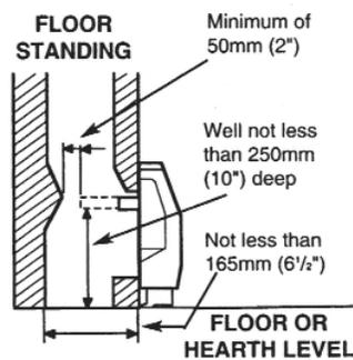
**1.8.2 Fitting to Pre-Fabricated twin wall metal Flue Boxes.**
