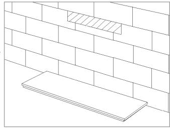
Remove all masonry from below the lintel, and clear debris from the cavity.
