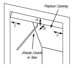
A.25mm down from top opening 25mm in from front of opening. C. Disregard outer 50mm either side of fireplace opening 16
