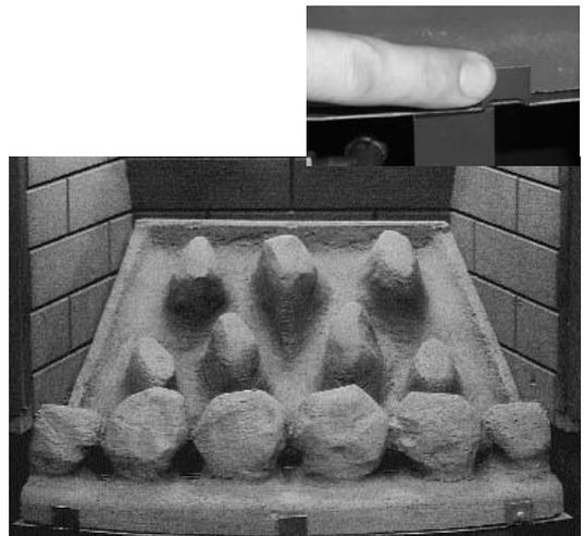
3. Open the bag of 16 moulded coals. All of the coals are the same. Take five coals and place them as shown. Care should be taken to ensure that the coals bridge the gap between the front coal and the four coal supports at the front of the matrix. Care should also be taken not to push the coals right down between the coal supports, as this can detract from the flame picture when the appliance is running.
