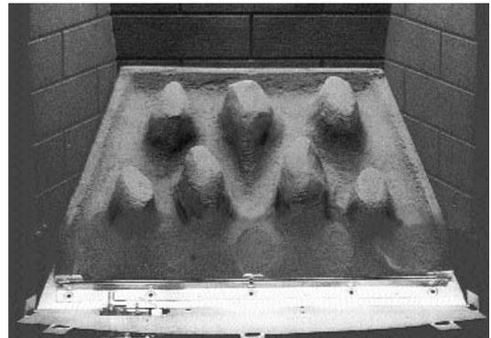
2. Next, remove the front coal strip from its protective packaging and position as shown. The rear edge of the front coal strip should fit in front of the burner rail. Again, do not place on top of the burner rails. When the front coal is in position bend up the three metal tags at the front of the tray to retain (inset).
