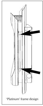
Non-concealed gas connections may be made using the entry points at either end of the firebox or the one in the bottom of the firebox. A concealed gas connection may be made using the knock out hole in the centre back of the firebox. Select the most appropriate entry point and knock out the relevant hole No more than 1.5m of 8mm diameter pipe must be used to avoid unnecessary pressure drops.
