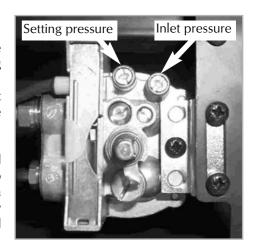
If the burner pressure is too low, then check the inlet pressure with the appliance running. If this is less than approximately 20mbar it will need to be reset by the gas supplier. If the setting pressure is too low, but the meter pressure is acceptable, then a problem in the supply pipework is to be suspected.
