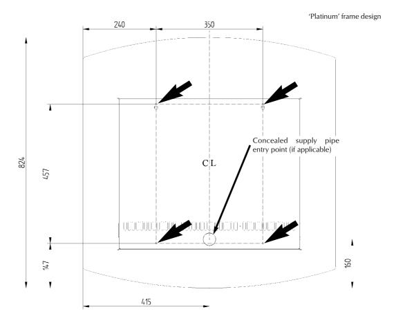
If the appliance is to be mounted on the inner leaf of a conventional cavity wall, or a solid wall, drill four holes using a 7mm masonary bit. Insert the fibre wallplugs provided.
