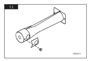
9.4 Reasemble in reverse order with correct aeration plate. NOTE: EVEN IF NO AERATION PLATE IS REQUIRED, THE SMALL SCREW MUST BE REPLACED.
