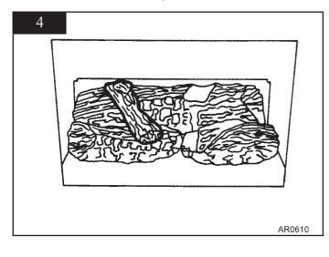
4.5 Place log E across from the rear of log A to log C on the right hand side. Again, there are cutouts for location. Log E should have the small branch on the right hand side when installed correctly. The front of the log should sit on the burner skin and should fit tight to log C. See diagram 5.
