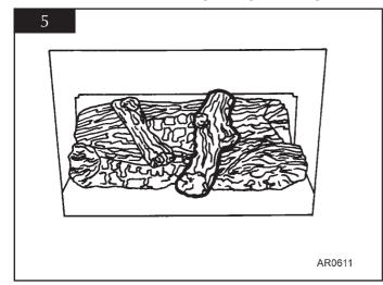
6.6 Place the embers along the front of the burner so as to cover the front edge. These can be placed up to the front edge of the burner ports. It does not harm the performance of the stove if these cover the burner ports but less yellow flames will evident. Place a few embers between logs B and C in the centre of the burner.
