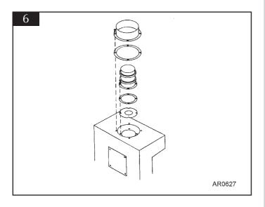
3.11 If the horizontal terminal is used assemble the required amount of vertical flue including the 90° elbow onto the stove. Drill through the fixing hole in the spigot using a 3.5mm drill and secure with the screw provided. Do not forget the optional decorative collar if you have purchased one. A wall plate is supplied to secure the flue to the inside wall. Bend the tab to 90° and loosely place on the elbow.
