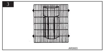
Any terminal which is less than 2 meters above any access (level ground, balcony or above a flat roof to which people hae access), is to be fitted with the guard supplied, see diagram 3.
