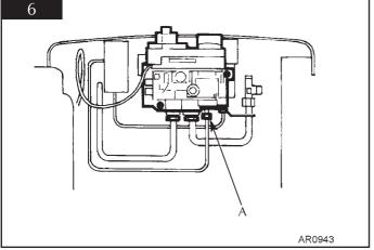
3.7 To remove the gasket, disconnect all the above components and withdraw the gasket. If it is damaged, replace with a new item. Always replace the gasket first when reassembling the pilot components.
