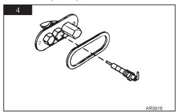
3.6 To remove the thermocouple, undo the retaining nut and withdraw the thermocouple, see diagram 5. Undo the thermocouple from the back of the gas valve, see diagram 6, arrow a. Reassemble in reverse order, do not overtighten.
