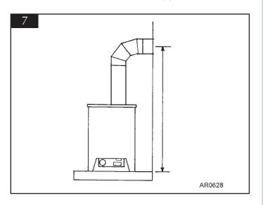
3.12 To determine the height of the hole for the horizontal flue, measure from the hearth to the centre of the elbow. See diagram 7. Refer to 3.4 for methods of cutting the hole.
