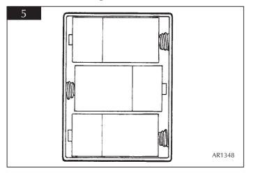
10.4 Push the battery holder back into its location and replace the front as detailed in the instructions supplied with the front.
