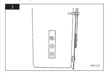
2.10.1 Press the ON / OFF button (2) once and the red LED will flash. The pilot will now light. This should take about 10 seconds
