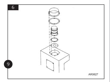
3.11 If the horizontal terminal is used assemble the required amount of vertical flue including the 90° elbow onto the stove. Drill through the fixing hole in the spigot using a 3.5mm drill and secure with the screw provided. Do not forget the optional decorative collar if you have purchased one. A wall plate is supplied to secure the flue to the inside wall. Bend the tab to 90° and loosely place on the elbow.
