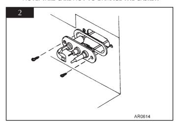
3.4 To remove the pilot injector, undo the compression nut on the pilot feed pipe and withdraw the injector which will be hooked onto the olive. When replacing an injector always make sure it is hooked onto the olive before inserting it into the pilot burner. See diagram 3.
