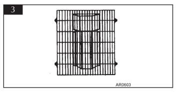
Any terminal which is less than 2 meters above any access (level ground, balcony or above a flat roof to which people hae access), is to be fitted with the guard supplied, see diagram 3.
