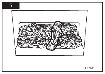
4.6 Place the embers along the front of the burner so as to cover the front edge. These can be placed up to the front edge of the burner ports. Do not cover the Burner ports. Do not place embers between Burner ports and pilot. Place a few embers between logs B and C in the centre of the burner.
