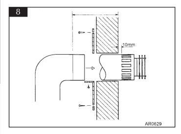
3.15 Once the length of the terminal has been obtained, mark the flue all the way round, insert the cardboard fitment as shown in diagram 9. This will support the inner flue. When cutting take care not to damage the edges of the flue. File any sharp edges from the cut end of the flue. REMOVE ANY CARDBOARD FITMENT REMAINING.
