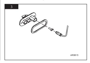
3.5 To remove the electrode, disconnect the ignition lead and undo the retaining nut. The electrode can now be removed, note the orientation of the electrode terminal when reassembling. See diagram 4.
