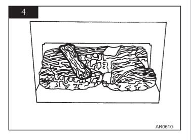
4.5 Place log E across from the rear of log A to log C on the right hand side. Again, there are cutouts for location. Log E should have the small branch on the right hand side when installed correctly. The front of the log should sit on the burner skin and should fit tight to log C. See diagram 5.
