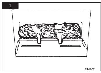
Place log B on the left hand side of the burner with the location bar on the underside of the log fully located in the long slot of the burner. Make sure the log is as far to the left as possible. See diagram 2.
