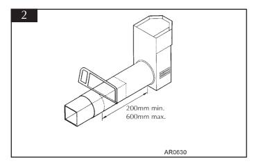
3.6 From outside, locate the flue assembly into the hole until the terminal is flat against the wall. Ensure the terminal is vertical. NOTE THE ORIENTATION OF THE TERMINAL. See diagram 4. Mark the four fixing holes, remove the terminal and drill the holes, inserting the rawplugs supplied.
