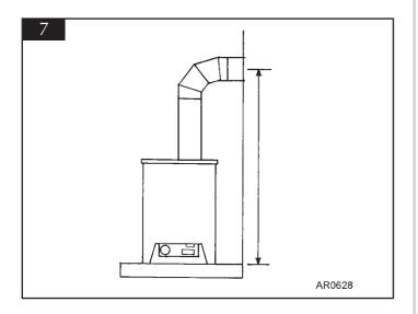
3.12 To determine the height of the hole for the horizontal flue, measure from the hearth to the centre of the elbow. See diagram 7. Refer to 3.4 for methods of cutting the hole.
