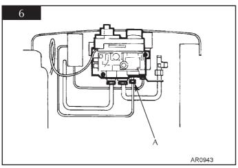
3.7 To remove the gasket, disconnect all the above components and withdraw the gasket. If it is damaged, replace with a new item. Always replace the gasket first when reassembling the pilot components.
