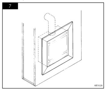
5.4.8 A removable access hatch must be left in the side of the chimney breast for future servicing and inspection of the appliance.
