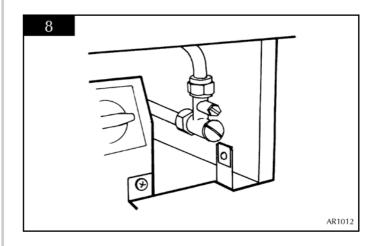
3.13 Connect a suitable pressure gauge to the test point located on the inlet fitting and turn the gas supply on. Light the appliance and check for leaks. Turn the appliance to maximum and check that the supply pressure is as stated on the databadge. Turn the gas off and replace the test point screw, turn the gas on and check the test point for leaks.
