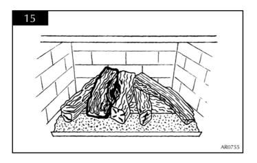
4.8 Place log 7 on the vermiculite at the front of the fire between logs 4 and 5. DO NOT PLACE THIS LOG ON THE BURNER. IT IS ONLY TO FILL THE GAP BETWEEN LOGS 4 AND 5. The charred effect should face the rear of the fire. See diagram 16.
