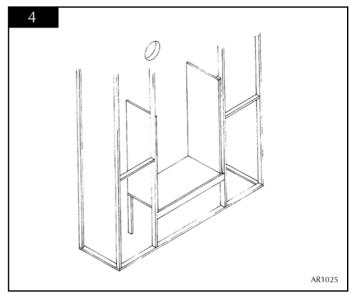
5.4.5 Place the cassette into position and fit a non-combustible panel above the cassette as shown. See diagram 5. Ensure the void is adequately ventilated.
