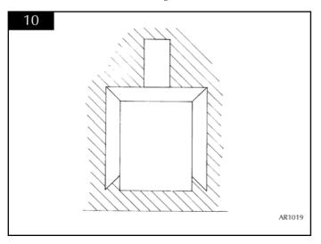
NOTE: In order to prevent possible plaster cracks, it is recommended to cover the immediate area above the cassette with non-combustible material such as marble or granite.
