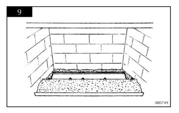
4.2 Place log 1 (large black log) on the burner. Ensure the rear of the log touches the rear of the burner. See diagram 10.
