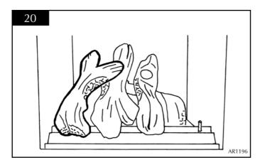
4.13 Place log E on to the last stud. The recess on the underside of the log should locate on to the top of log D. See diagram 21.
