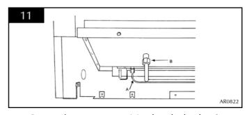
6.3 Remove the two screws retaining the valve bracket. See diagram 12.
