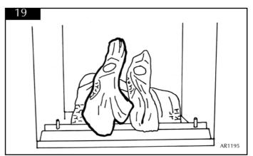
4.12 Place log B on the first stud. The recess on the underside of the log should locate on to the top of log C. See diagram 20.
