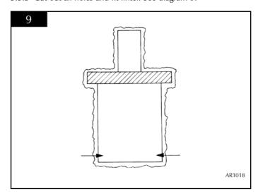
5.5.4 Apply plaster finishing around the aperature that the cassette will fit into. See diagram 10.
