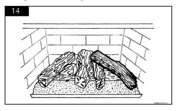
4.7 Place log 6 on the remaining stud and lean the log on to log1 between logs 2 and 3. There is a notch to locate the log.See diagram 15.
