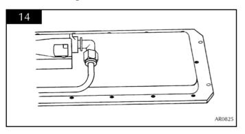
8.2 Rotate the injector until it is fully removed, and install the correct replacement injector. Re-assemble and turn the gas supply on, check for any leaks.
