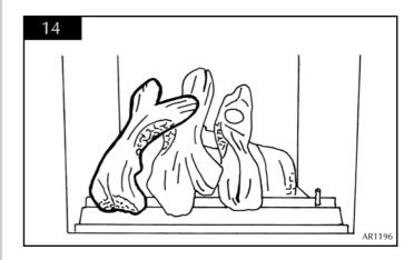
6.13 Place log E on to the last stud. The recess on the underside of the log should locate on to the top of log D. See diagram 15.
