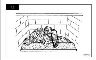
4.6 Place log 5 on top of log 4 and ensure the two large locations engage. Locate the front of the log on to the far right hand stud. See diagram 14.
