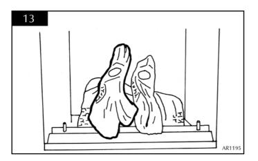
6.12 Place log B on the first stud. The recess on the underside of the log should locate on to the top of log C. See diagram 14.
