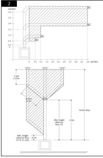
TAKE CARE WHEN MARKING OUT FOR THE FLUE AS IT IS DIFFICULT TO MOVE AFTER INSTALLATION. IF A RESTRICTOR IS REQUIRED FIT THIS BETWEEN THE SMALL OUTLET SPIGOT AND THE AIRDUCT SEE DIAGRAM 3. REFER TO TECHNICAL SPECIFICATIONS FOR RESTRICTOR SIZE.
