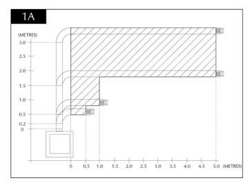
Start of bend to centreline of horizontal flue 170mm. Centreline of vertical flue to end of bend 220mm.
