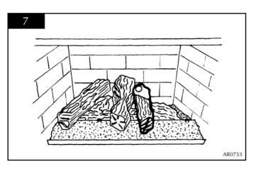
6.6 Place log 5 on top of log 4 and ensure the two large locations engage. Locate the front of the log on to the far right hand stud. See diagram 8.
