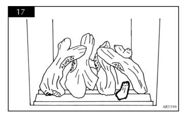
6.16 With the granules fill the front compartment around the logs evenly. ENSURE NO GRANULES FALL ON THE BURNER. See diagram 18.
