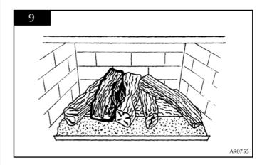
6.8 Place log 7 on the vermiculite at the front of the fire between logs 4 and 5. DO NOT PLACE THIS LOG ON THE BURNER. IT IS ONLY TO FILL THE GAP BETWEEN LOGS 4 AND 5. The charred effect should face the rear of the fire. See diagram 10.
