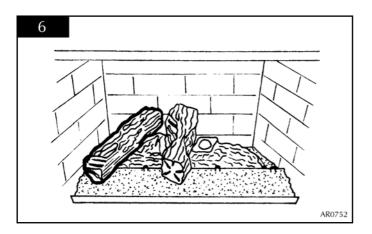
6.5 Place log 4 on the right hand side of the centre log. There is a large recess on the underside of the log, which locates on log 1. See diagram 7.
