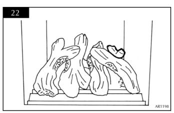
4.15 Place log G at the front of the fire between logs D and E. DO NOT PLACE THIS LOG ON THE BURNER. IT IS ONLY TO FILL THE GAP BETWEEN LOGS D AND E. The charred effect should face the rear of the fire. See diagram 23.
