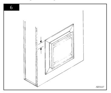
5.4.7 Push the cassette back into its final position and connect the flue system, gas and electric services using the openings in the side of the chimney breast for access. Following commissioning complete the sides of the chimney breast. See diagram 7.
