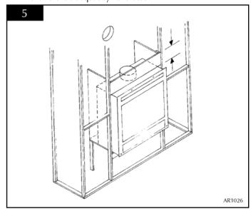
5.4.6 With the cassette forward of its final position apply plasterboard to the front of the chimney breast and apply plaster finish. In order to prevent possible plaster cracks, it is recommended to cover the face of the wall immediatly above the cassette with non-combustible material such as marble or granite. See diagram 6.
