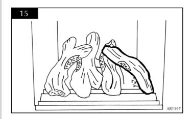
6.14 Place log F resting on the rear tray and leaning forward to locate in the recess in log E. See diagram 16.
