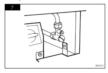
c) Disconnect the external pilot pipe from the brass fitting. See diagram 8, arrow A.
