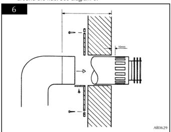
A wall plate is supplied to secure the flue to the wall. Bend the tab to 90 . Assemble the plate onto the flue but only secure to the wall and flue when the flue is fully assembled. See diagram 6.
