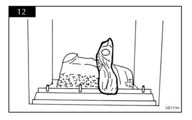
6.11 Place log C on the second stud and resting at the rear on log A. See diagram 13.
