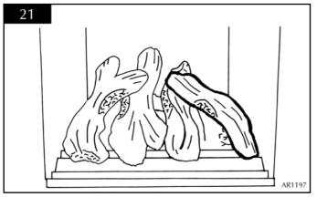
4.14 Place log F resting on the rear tray and leaning forward to locate in the recess in log E. See diagram 22.
