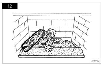
4.5 Place log 4 on the right hand side of the centre log. There is a large recess on the underside of the log, which locates on log 1. See diagram 13.
