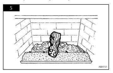
6.4 Place log 3 on the far left-hand stud. The recess on the underside of the log should locate on the top of log 1 on the far left-hand side. See diagram 6.
