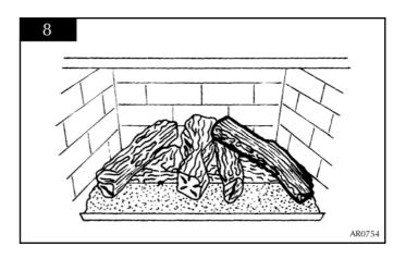
6.7 Place log 6 on the remaining stud and lean the log on to log 1 between logs 2 and 3. There is a notch to locate the log. See diagram 9.
