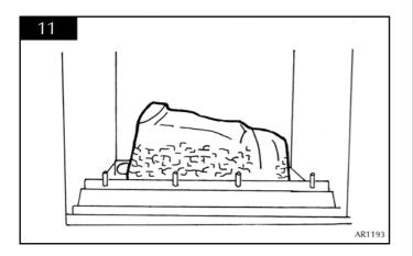
CENTRALISE THE LOG BETWEEN THE BURNERPORTS AT EITHER END.
