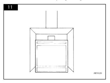
5.5.6 Raise the cassette into its final position and support it on 12mm thick non-combustible material. See diagram 12.
