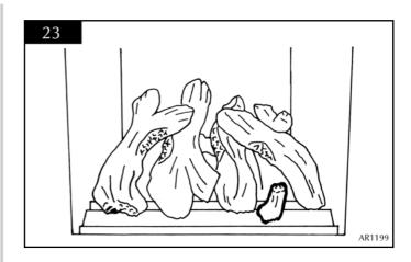
4.16 With the granules fill the front compartment around the logs evenly. ENSURE NO GRANULES FALL ON THE BURNER. See diagram 24.
