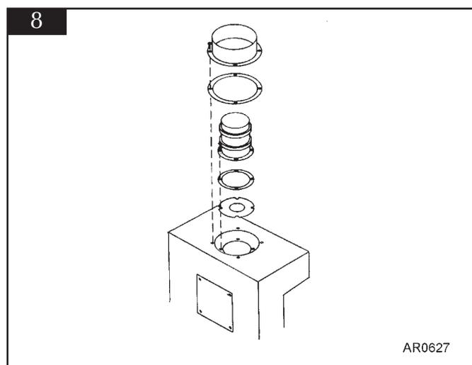
3.13 When fitting the top flue it will be necessary to open the second cavity containing the casing, and place the top casing ring and grill on to the top of the unit and place the first flue length through them in to the spigot and optional decorative collar, part no 8548 to cover the gap between the top plate and the flue if required.
