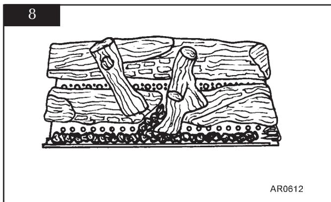
**NOTE: ENSURE THAT LOGS ARE POSITIONED, AS DETAILED ABOVE.**
