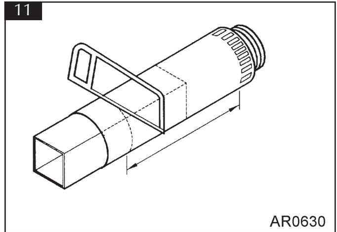
3.19 Remove the stove and flue assembly from the hearth and drill the four fixing holes for the wall plate, insert the rawlplugs supplied. Assemble the horizontal flue onto the elbow and reposition the stove ensuring the flue slides smoothly through the wall. alternatively, place the flue terminal in the wall, place the stove on the hearth and connect the flue to the elbow. Reposition the stove.
