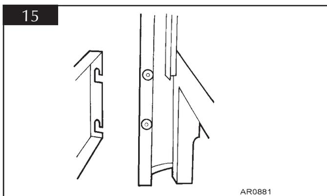
3.25 Place the steel top onto the casing so that the 2 lugs on the underside locate the top centrally within the casing. Place the cast iron grille into the recess in the centre of the top panel and locate the blanking plate into the grill (if required). See diagram 16.
