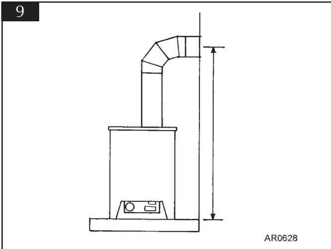
3.16 The final length of horizontal flue pipe incorporates the terminal. This is the only section that can be shortened.
