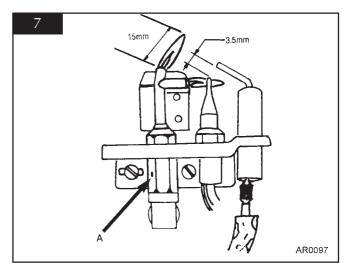
6.6 After reassembly, check for gas soundness and carry out a flame failure functional check details in the flow chart, especially the mag drop out time.
