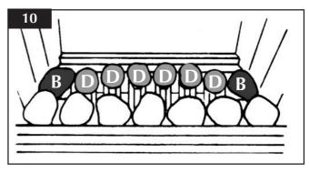
7.16 Place 5 oval pebbles (marked B) at the back of the flame baffle as shown in diagram 11.
