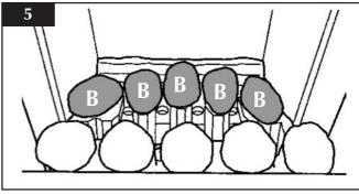
7.11 Place 3 oval pebbles (marked B) at the back of the flame baffle as shown in diagram 6.
