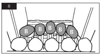
5.8 Place 3 oval pebbles (marked B) at the back of the flame baffle as shown in diagram 9.
