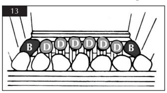
5.13Place 5 oval pebbles (marked B) at the back of the flame baffle as shown in diagram 14.
