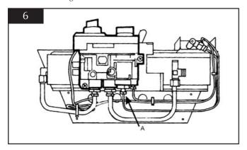
6.5 Replace with a new pilot assembly, set the spark gap. See diagram 7.
