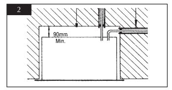
4.3 Remove the fire assembly (see diagram 3), and offer the convector box into the opening, checking that it fits squarely. Mark the fixing holes and the gas pipe entry positions. See diagram 4.
