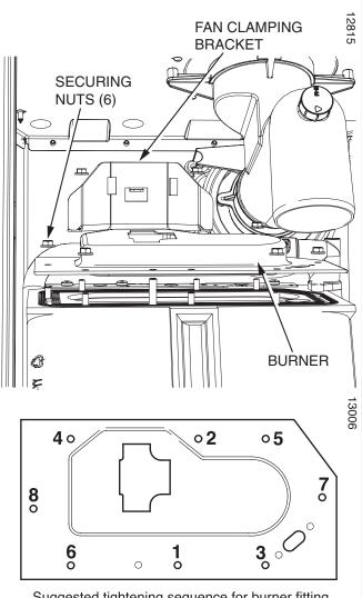
Suggested tightening sequence for burner fitting
