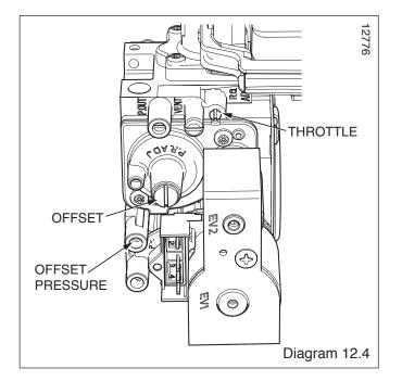
A competent person should only carry out any adjustment to the gas valve, refer to diagram 12.4.
