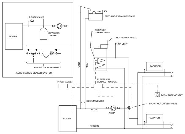
OPEN SYSTEM WITH FEED AND EXPANSION TANK
