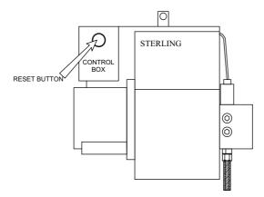
The burner is equipped with a flame failure device, when activated the reset button on the burner control box is illuminated. Refer to the fault finding section of the handbook to identify possible causes.
