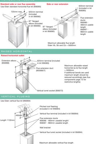
Maximum allowable vertical flue length (using extension ducts) Eden Vb, Sb and Cb = 6000mm
