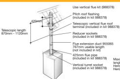
Maximum allowable vertical flue length (using extension ducts) Hero 30-75 = 4000mm Hero 90 = 3200mm
