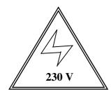
**Warning High Voltage!** This sign is located on the back of the control box housing warning of high voltages within the control box. Turn off and isolate the appliance before removing this cover.
