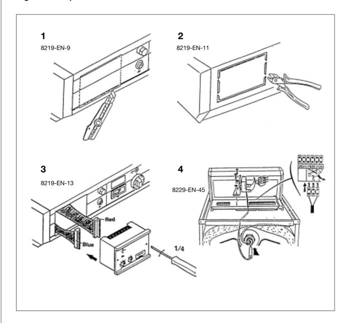
The SVR option box is to be fitted in the front part of the control panel. To do this:
