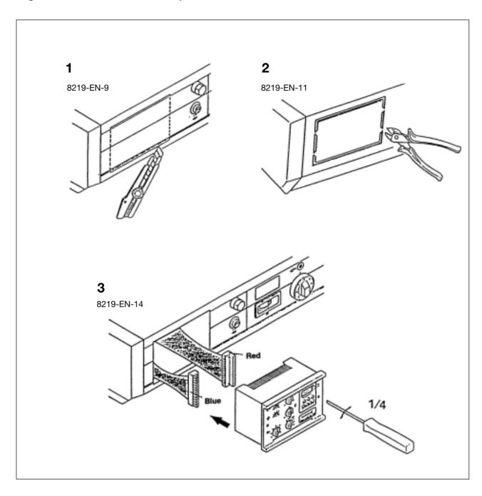
The SV-matic weather compensator is fitted in the front part of the control panel. To do this:
