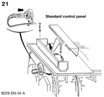
Fix the control panel at the rear, on the top panel using 2 self tapping screws dia. 3.94x25 + lock washers.
