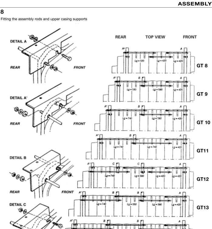
Fit the upper assembly rods (body accessories pack) in the order given in the figure above. Place the expansion spring and its washer on each rod towards the rear. Stop tightening the nuts when the free space between the threads is about 2 mm.
