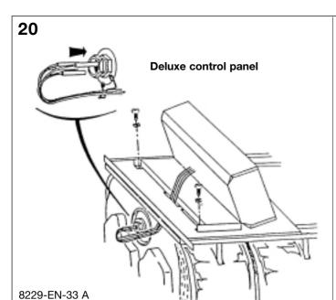
Screw the control panel at the front on the top panel using 2 self tapping screws dia. 3.94x12.7 + lock washers.
