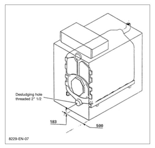
A desludging hole of  $\emptyset$  1"1/2 supplied with a plug is provided in the lower part of the boiler to enable sludge to be drained out. The installer can fit 1/4 turn valve.
