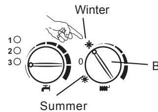
3. The boiler will commence the ignition sequence. The green operational light 1 (E) indicates boiler running for central heating.
