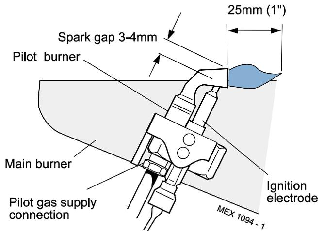
5. Undo the gas cock union. Remove the 4 wing nuts and withdraw the burner and controls assembly, complete, from the boiler.
