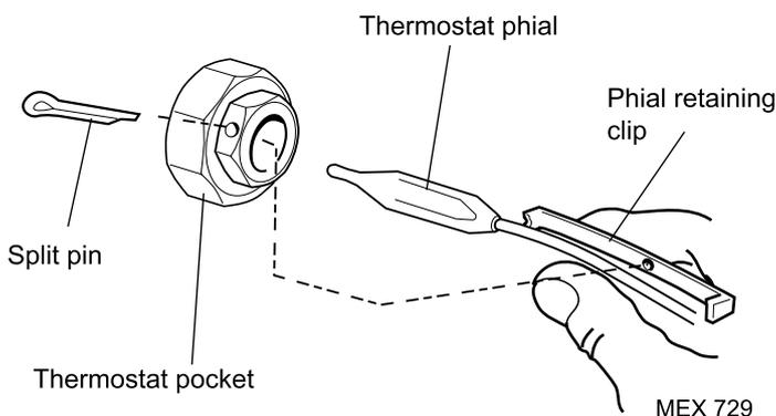
8. Insert the thermostat phial and phial retaining clip into the thermostat pocket. Take care not to kink the thermostat capillary as it is unwound and secure it with the split pin, as shown.
