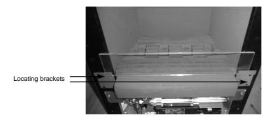
d) Locate the front section onto the retaining brackets as shown below in Fig. 16
