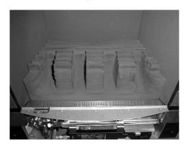
Position front ceramic rail on burner front ceramic support and ensure that the locating channel in the front ceramic rail is correctly located onto the lip on the burner front ceramic support. (See fig. 14 below)
