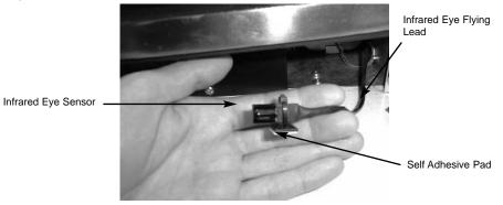
Remove the backing paper from the self adhesive pad and position the infrared eye in the air channels in the ashpan cover, so that the infrared eye is flush with the front edge of the ashpan cover, as shown below in Fig. 19. Check the operation of the handset, as detailed in Section 3.3 and adjust the position of the infrared eye if necessary.
