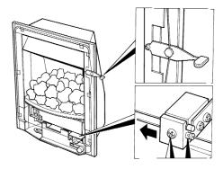
Unscrew the burner assembly fixing screws at either side of the firebox, and the two fixing screws at the base of the fire (See fig. 7 below). Carefully pull the base of the burner forwards from the fuel-bed support panel. The burner can now be removed from the appliance.
