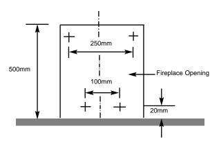
Fit the wallplugs provided and screw the fixing eyes securely into the rear of the fire opening. If the clearance at the rear of the fire is at the minimum specified for a precast flue application, it may be necessary to bend over the lower fixing eyes after screwing them fully in to the rear of a pre-cast starter block.
