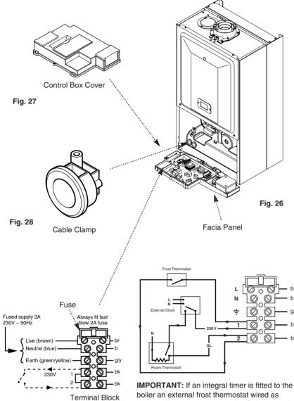
**IMPORTANT:** If an integral timer is fitted to the boiler an external frost thermostat wired as shown will not operate correctly. Only external timers may be used in such installations, as in the diagram.
