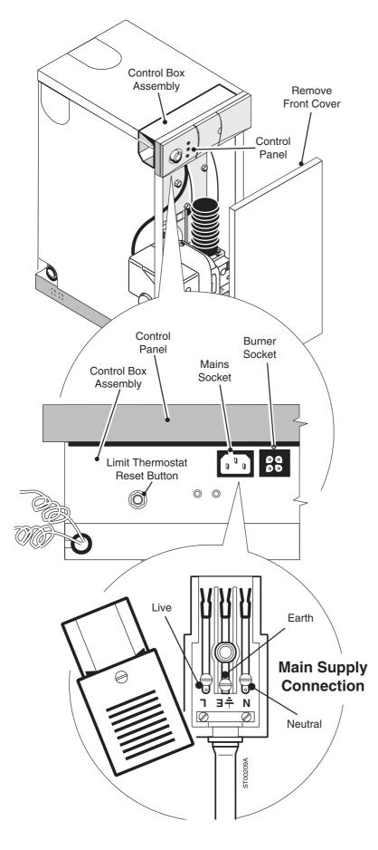
**Wiring Diagrams:** Refer to wiring diagrams in Section 1 of these Instructions. The mains inlet plug is provided in the bag of fittings supplied.
