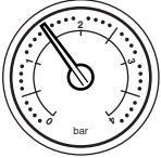
Fig. 13 Normal Pressure (operating)
