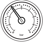
Fig. 19 Normal Pressure (operating)
