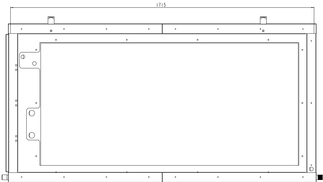
Figure 7.2 : Max. dimension cooling coil 1705mm
