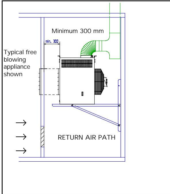
A return air grille must be provided to ensure that an unobstructed path for re-circulation; air back to the air heater is maintained, this is to ensure that a negative pressure cannot develop within the space where the air heater is installed.
