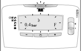
• Warning: Take care not to overfill the boiler. At a pressure of 2.5 bar or above the high system water pressure fault will be displayed. The pressure must be reduced to 1.0 bar by opening the drain valve, see diagram 1. If the fault continues call your Installation/Servicing company or Heatcall using the telephone number on the inside front cover of this literature.
