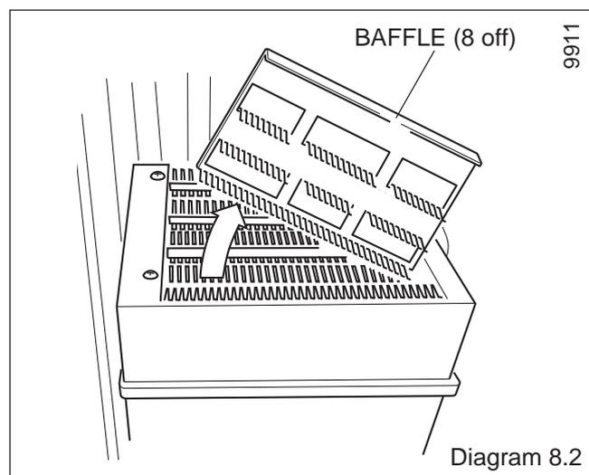
Clean the heat exchanger flueways with a suitable stiff brush.
