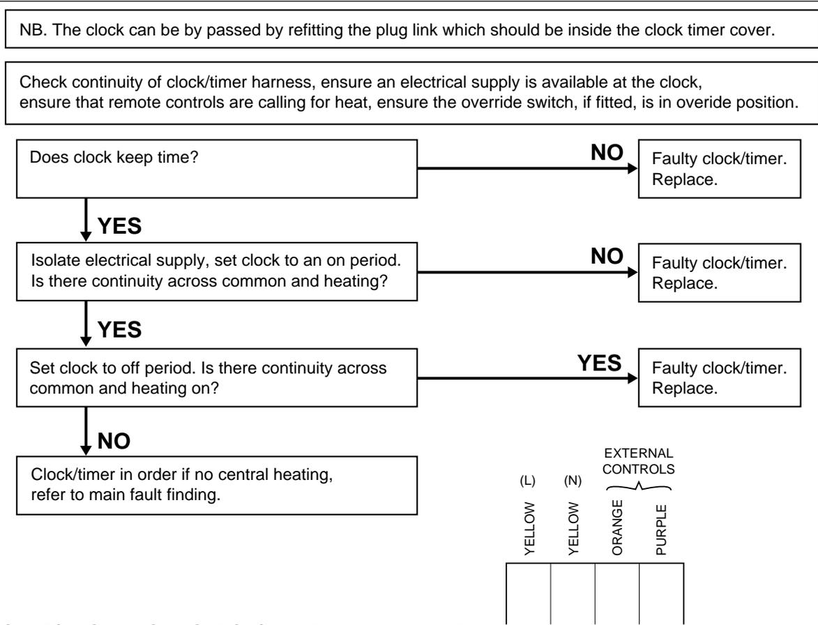
**ELECTRO/MECHANICAL CLOCK/TIMER FAULT FINDING**
