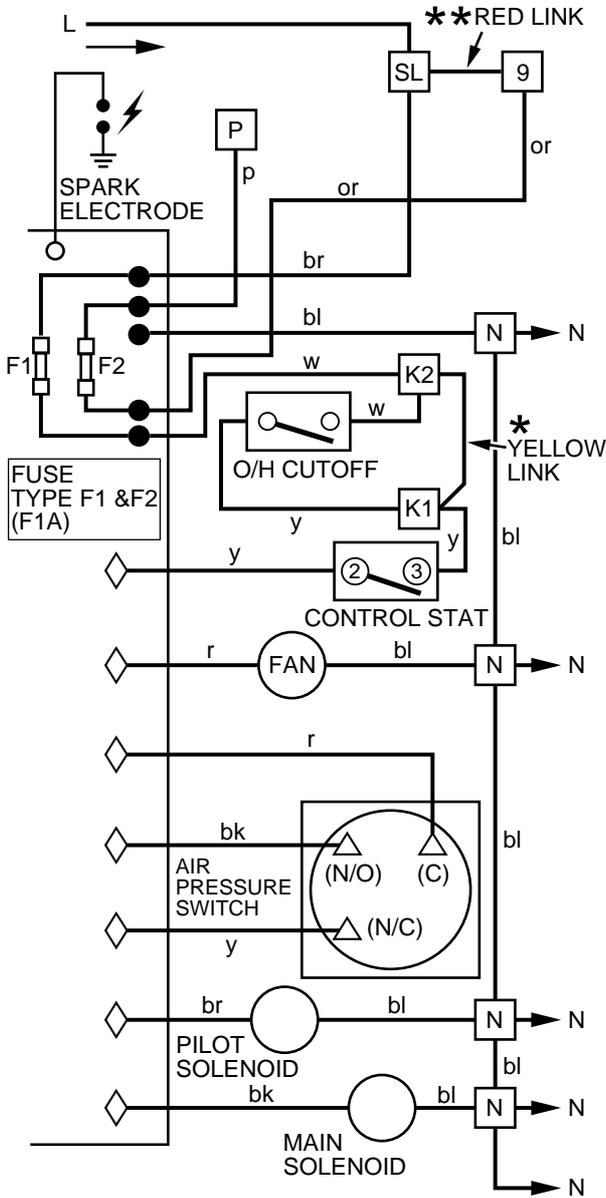
**\* Yellow Link fitted to bridge out the overheat cutoff**
