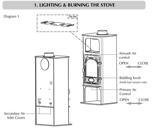
N.B: The secondary combustion air control at the rear of the stove is pre-set during manufacture.
