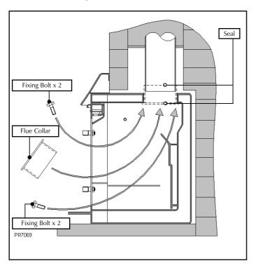
4.5 Should the Stockton convector be installed on an unlined, masonry flue first fit a non-combustible closure/register plate to locate first section of single wall fluepipe from the Stockton convector to the old system. Then make the collection as with a flue liner system. Do not connect the system into large voids that could exist in older chimney systems. If this is the case consider using a flue lining system to improve the Stockton convector operation.
