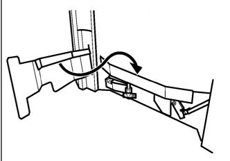
Figure 36. Fitting the burner baffle (**Dream model only**)
