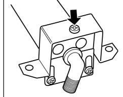
Figure 61. Main burner injector removal
