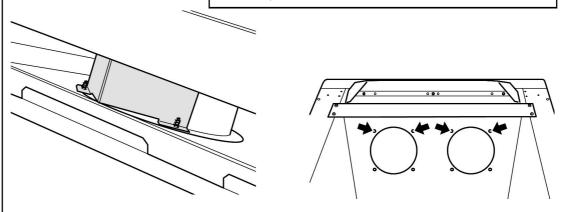
Figure 14. Fitting port covers to 'Icon' model.
