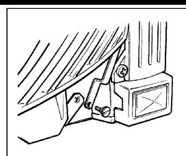
Figure 39. Control bar and pivot bracket (Shown with "Adorn")
