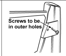
Figure 42. Casting screw position
