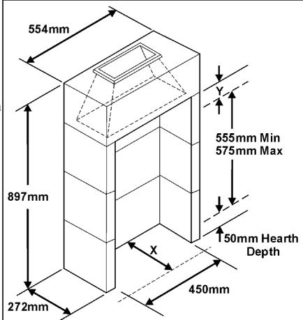
Dimension 'X' to be 240mm minimum. This will be made up of 220mm starter block depth plus at least 20mm of non-combustible fireplace material (Plaster, marble, etc).
