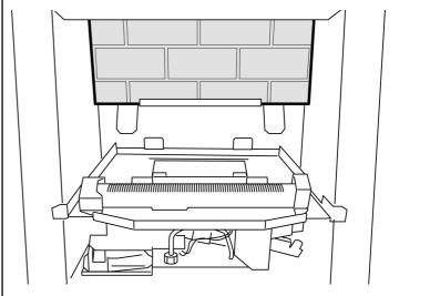
Figure 28. Ceramic rear wall installation
