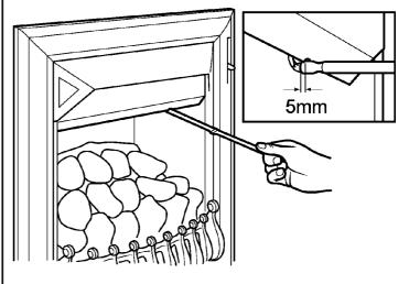
Figure 45. Smoke match tube position (Shown with 'Visage' fascia)
