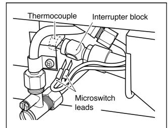
Figure 49. Thermocouple interrupter block
