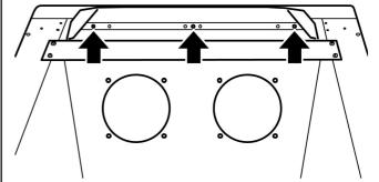
Figure 13. Fitting outlet baffle (The outlet baffle design may differ from that shown)
