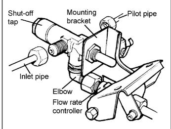
Figure 58. Shut-off tap (Viewed from rear with burner turned over)
