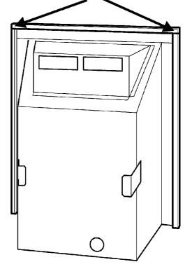
Figure 17. Fitting the foam seal
