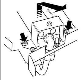
Figure 60. Removal of burner
