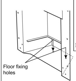
Figure 23. Floor fixing
