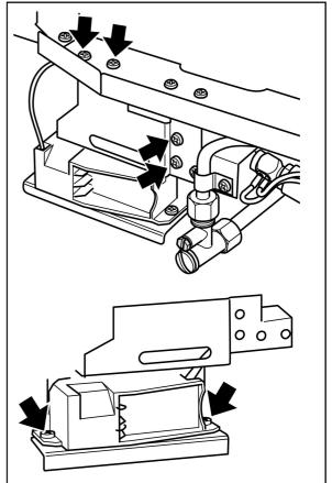
Figure 56. Removal of electronic generator
