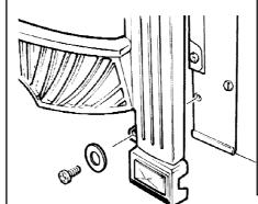
Figure 31. "Adorn" fascia bottom fixing.
