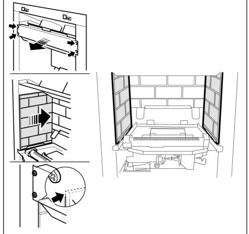
Figure 29. Ceramic side walls installation
