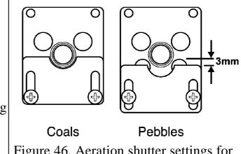
Figure 46. Aeration shutter settings for 'coal' and 'pebble' ceramic fuel effects.
