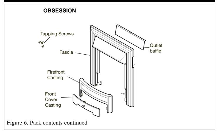
Carefully remove all the contents. Take special care in handling the ceramic pieces. Take care not to bend or distort the slide control linkage when handling the fascia. Check that all the listed parts are present and in good condition.
