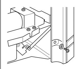
Figure 35. "Adorn" fascia bottom fixing.
