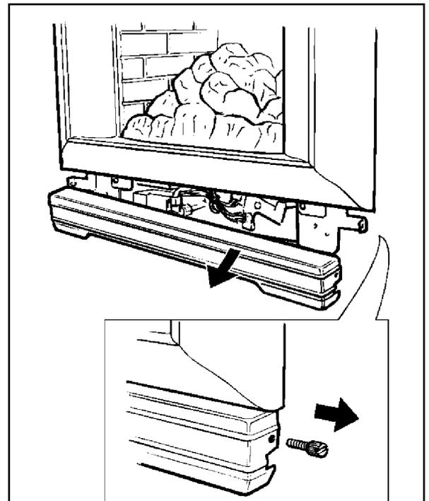
Figure 4. “Icon” bottom front cover removal.
