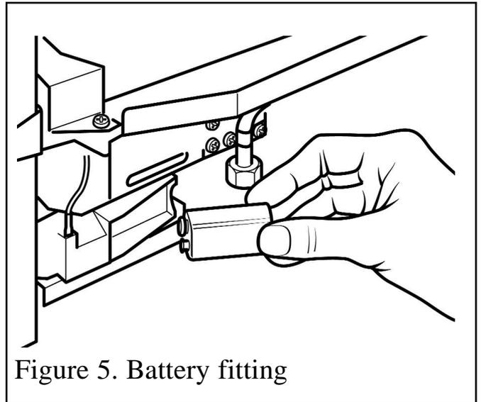
Figure 5. Battery fitting
