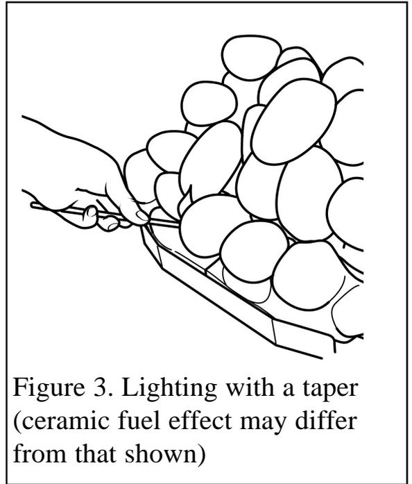
Figure 3. Lighting with a taper (ceramic fuel effect may differ from that shown)
