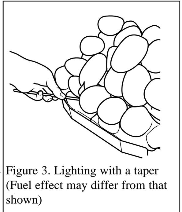
Figure 3. Lighting with a taper
