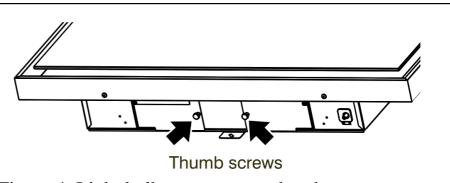
Figure 4. Light bulb access cover thumbscrews
