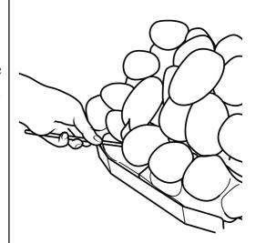
Figure 3. Lighting with a taper (ceramic fuel effect may differ from that shown)
