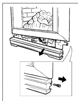
Figure 4. "Icon" bottom front cover removal.
