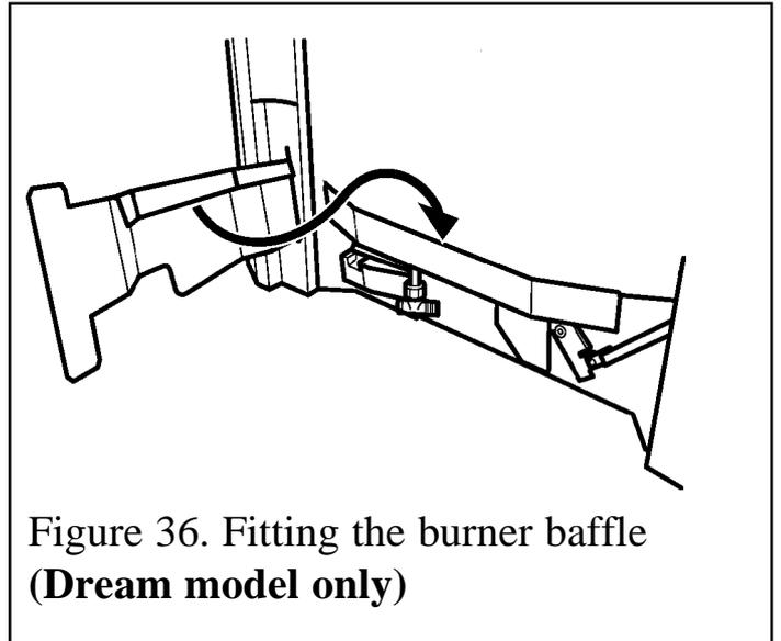
Figure 36. Fitting the burner baffle (Dream model only)
