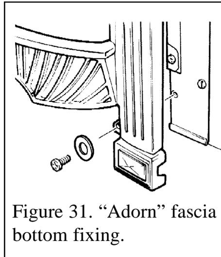
Figure 31. “Adorn” fascia bottom fixing.
