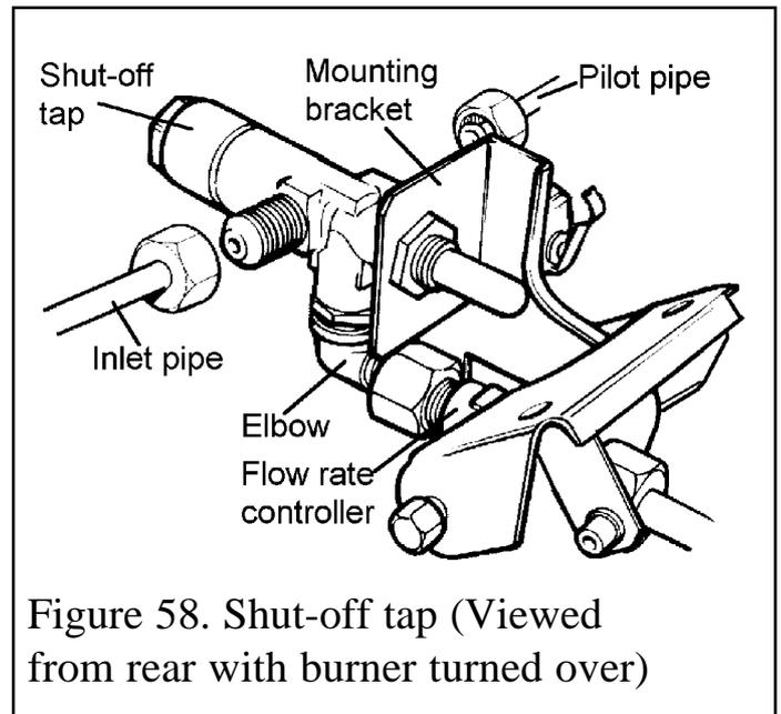
Figure 58. Shut-off tap (Viewed from rear with burner turned over)
