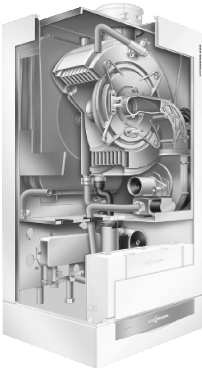
Figure 2/C: Sectional Diagram (Combi Boiler Illustrated)
